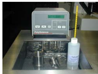
Bob, Cup and Test Fluid placed in a water bath conditioned to 25°C.
