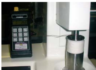
Damp cloth wrapped around the Bob, Cup and Test Fluid with microprobe thermocouple inserted reaching 25°C.
