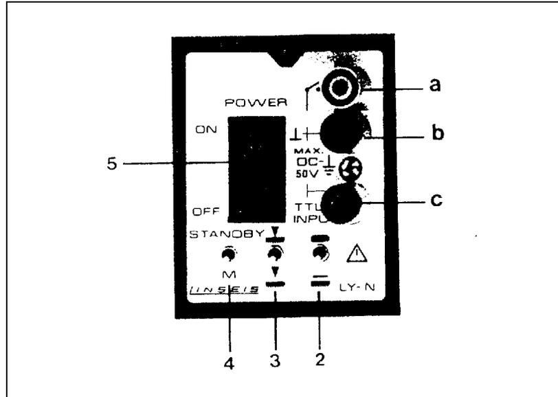
1. The input jacks a, b, and c are for external pen up/down control.
